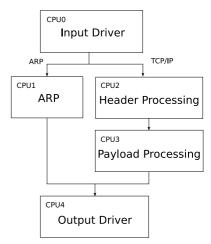
Figure 3: Pipelining and parallelizing a network stack.
